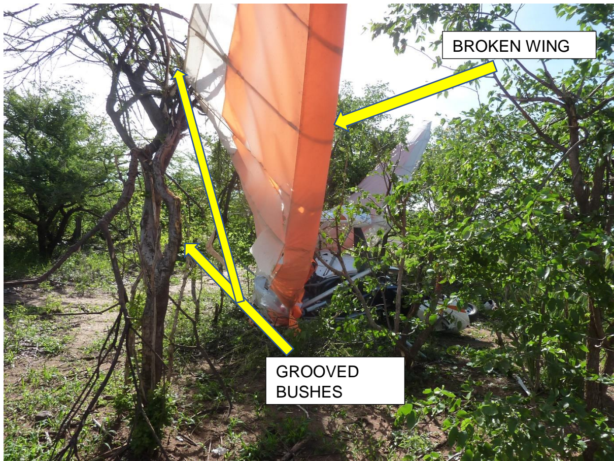
Fig.11: Microlight showing Broken Wing and Grooved Bushes
