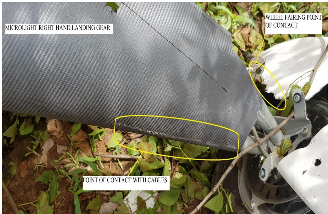
Fig 2: First point of contact and breaking of fairing
