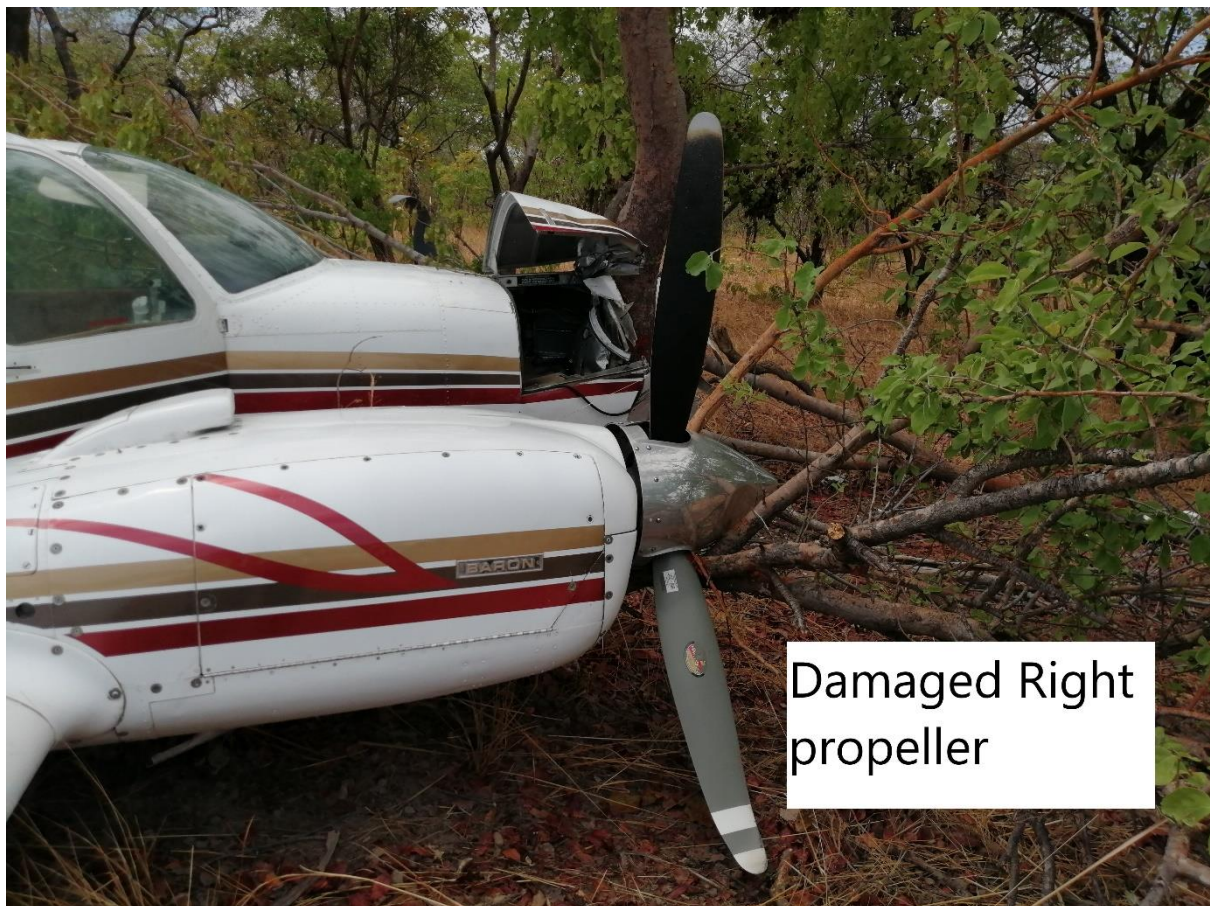
Fig. 1.2: Damaged Right Propeller
